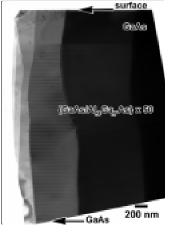
A Multiple Quantum Well structure grown by MBE showing the thickness terraces possible with a *MicroCleave*<sup>™</sup> sample. Image Courtesy of Scott Walck -Materials Directorate WPAFB. (Now with PPG Industries)
