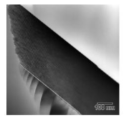
An X-ray mirror consisting of 45 layers of alternating Mo/amorphous Si (7.0nm period) on a Si substrate. Image courtesy of John McCaffrey - National Research Council of Canada.
