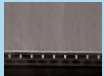
Fig 5: Same area like Fig 4 at an higher magnification, demonstrating surface smoothness and a fully intact interface.
