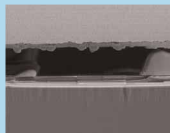
Fig 3; Completed cut after 3h of ion milling
