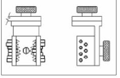
into a specially designed right angle holder. As there are no locating pins in this design, you can rotate the sample 360 degrees in both a horizontal and a vertical plane.
